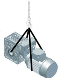
The eyebolt can lift just the gearbox and not the parts it will be attached to. Regarding gearboxes that weigh more than 30 kg not equipped with an eyebolt, a suitable eyebolt should be used to lift them in complete safety. Otherwise exercise extreme caution and use slings to lift the gearboxes. The types of eyebolts are given in the chart.
